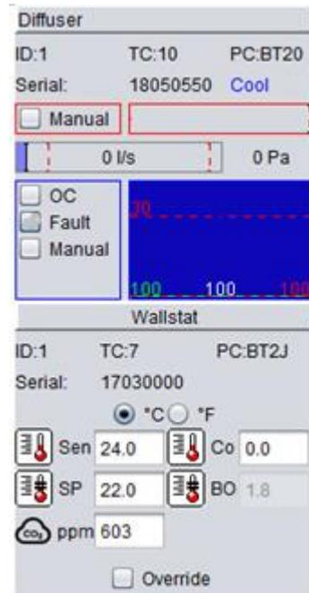
Wallstat LCD display: To select the CO2 for permanent display on the LCD, click on the wallstat icon and write in following two commands:
