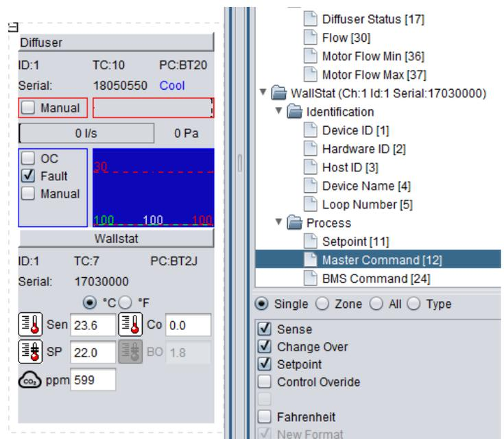
ii.    Select and run the CO2 wizard. Set the CO2 high and low thresholds. Press Apply.
