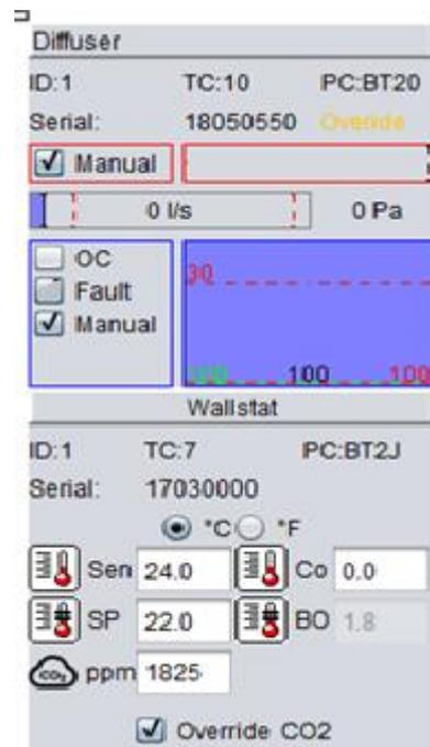
Once the CO2 level is reduced to below the CO2 low threshold, i.e. 700ppm, as set in our example, the diffuser control will revert to normal operation. Manual will be off.
